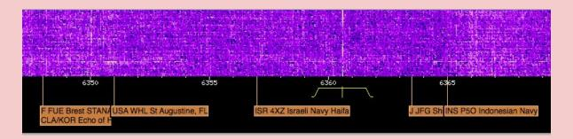
You have options to listen in modes adapted for CW (continuous wave / Morse code). You'll notice that your yellow cursor has a central line – the signal, and an upper and lower sideband. These switch if you change the options in this controller between single sideband transmissions (LSB for lower sideband and USB for upper sideband), AM (amplitude modulated) or FM (frequency modulated) transmissions. You may find it helpful to use the noise reduction filters on your dashboard.
